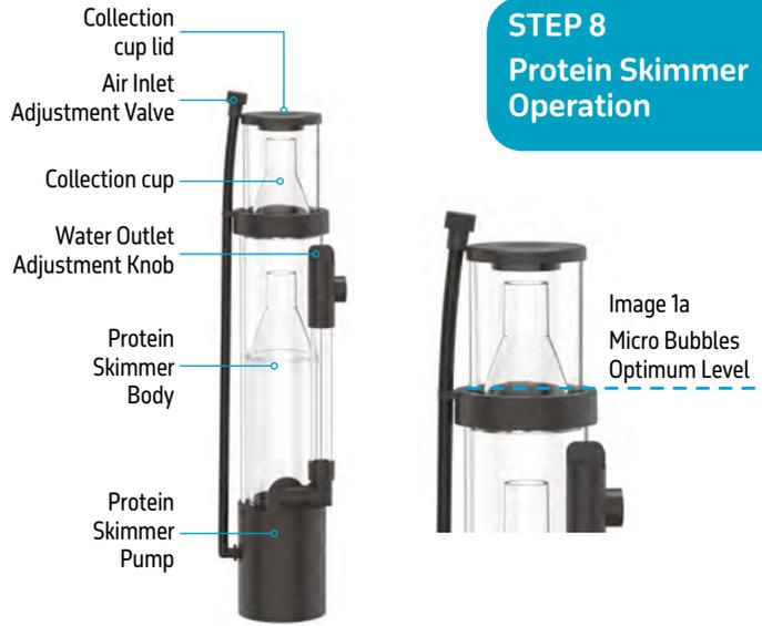
1. Ensure the protein skimmer collection cup and lid are securely and correctly positioned. Failure to do so could result in leaks.
