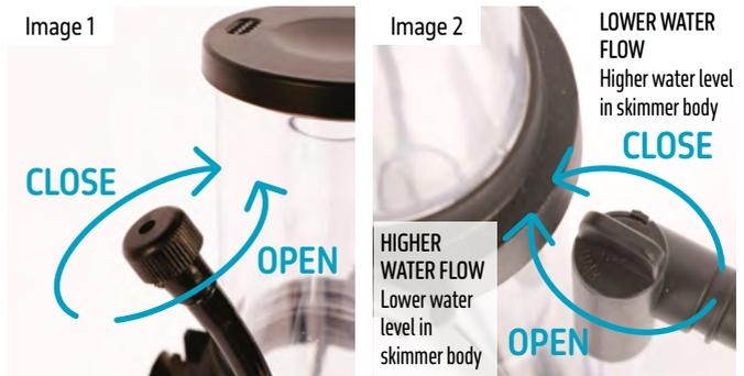
3. The water outlet adjustment knob can also be used to lower the water level (turning clockwise) or to raise the water level (turning anti-clockwise) see image 2.
